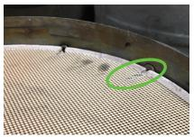
**Signs of Moved Substrate:** Substrate has shifted enough to touch the sensor ports or retaining ring.
