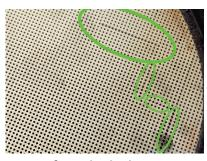
Signs of Cracked Filter: Dark straight lines that extend across multiple cells. This could be a single line or multiple lines connected forming squares.
